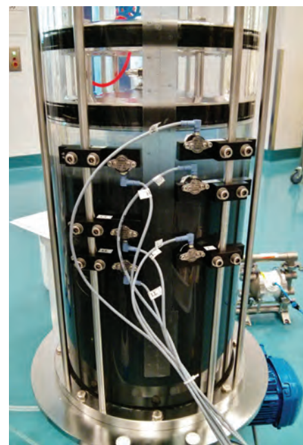
Rhobust ® Expanded bed absorption chromatography column displaying level control of the bed height.
