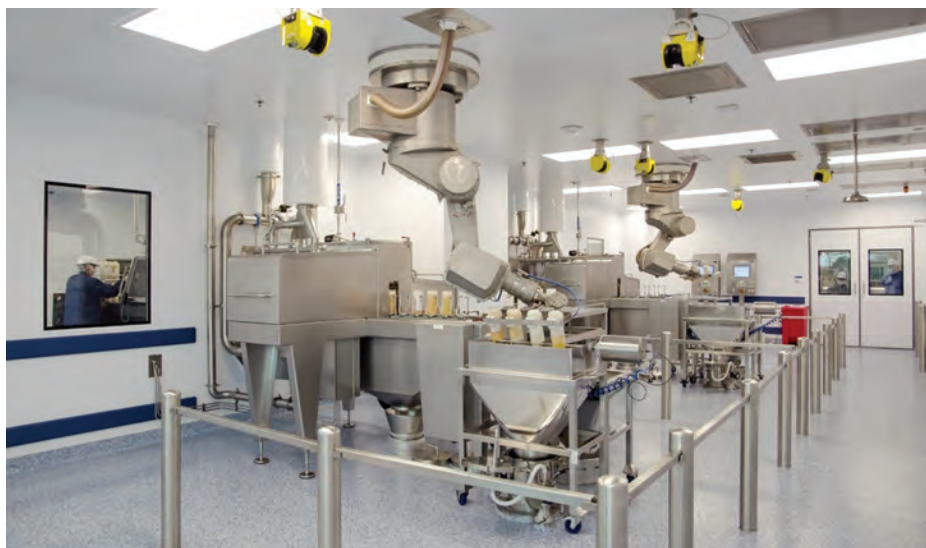
Automated bottle opener - robotics prevent human interaction and potential contamination.
