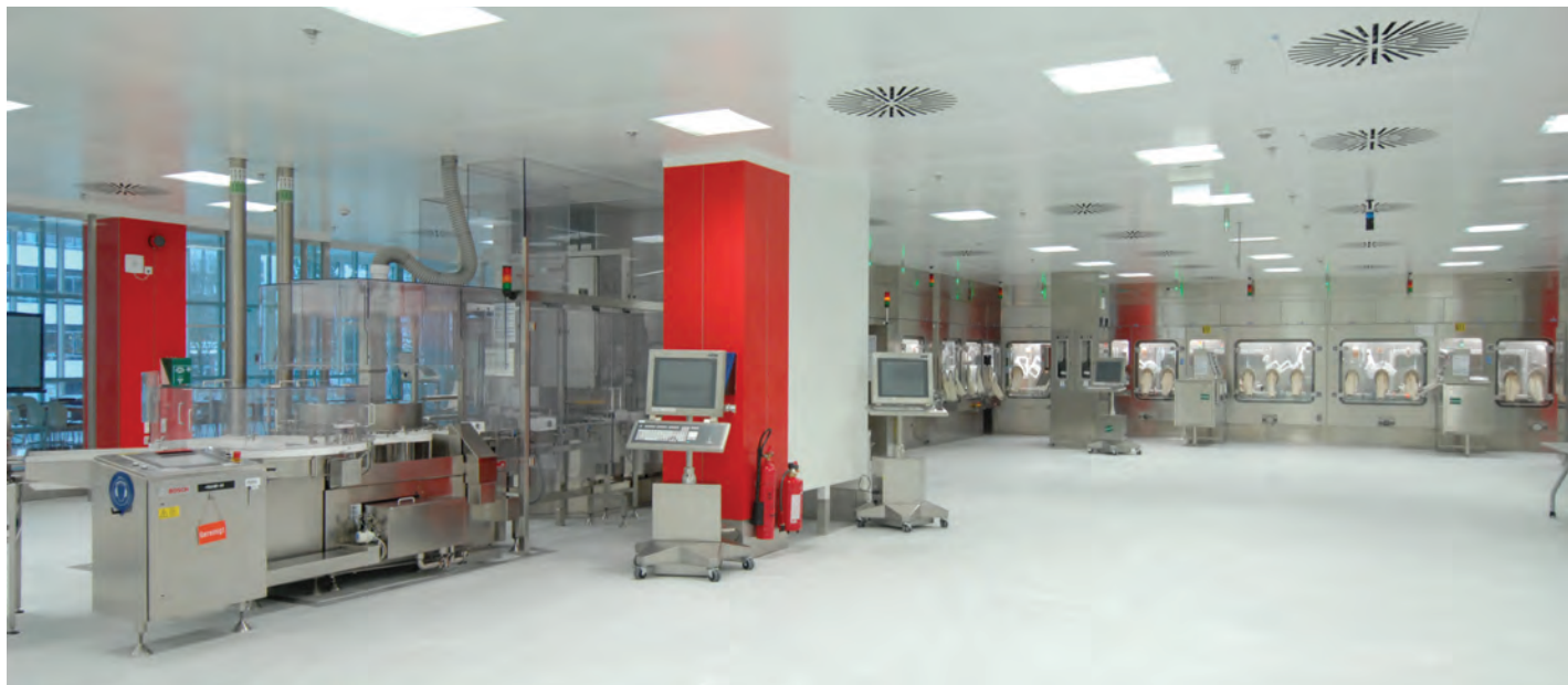
Vial filling with automatic loading and unloading units.
