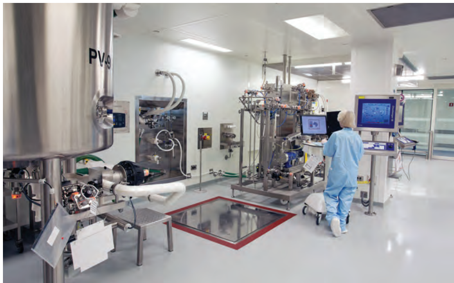
Technician interaction with Electronic Batch Records (EBRs) using Human Machine Interface (HMI).
