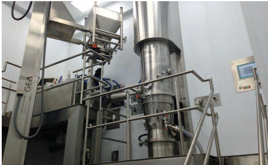
Fully contained product transfer in large scale granulation.
