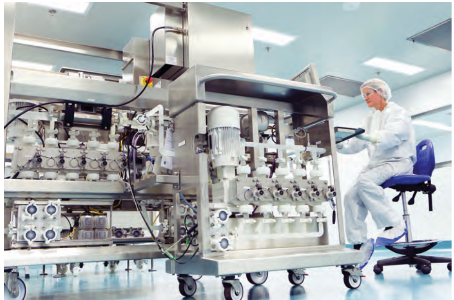
Chromatography system with inline dilution and buffer conditioning capacity.
