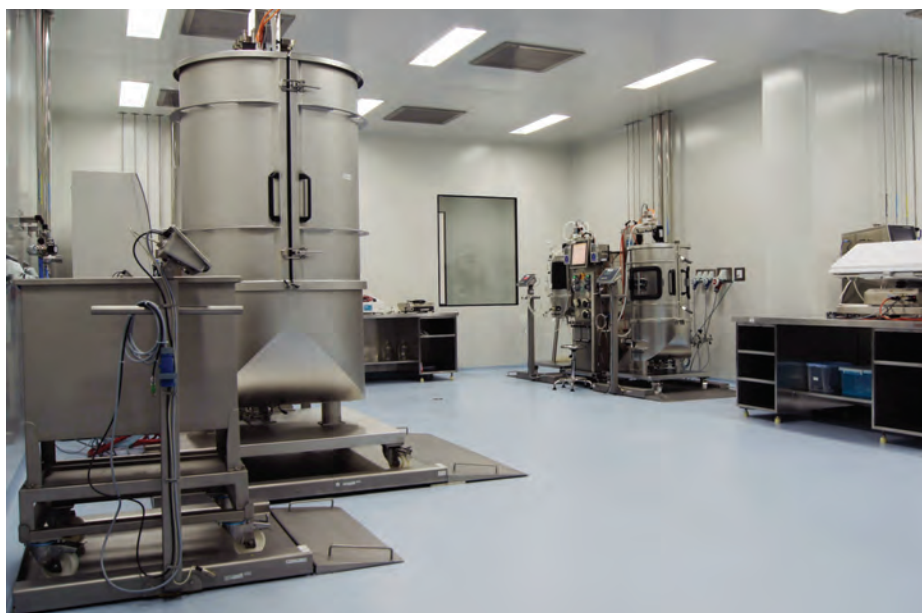
Cell culture 50 L / 200 L / 1000 L bioreactor line.
