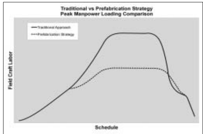
Figure 7. Prefabrication on Strategy Impact on Site Labor Requirements - This demonstrates the reduction in peak site labor forces associated with a prefabrication approach using conventional building construction. The reduction in the peak is a reflection of the reduced requirement for process, mechanical, electrical, instrumentation and control, and architectural trades on the project site.
