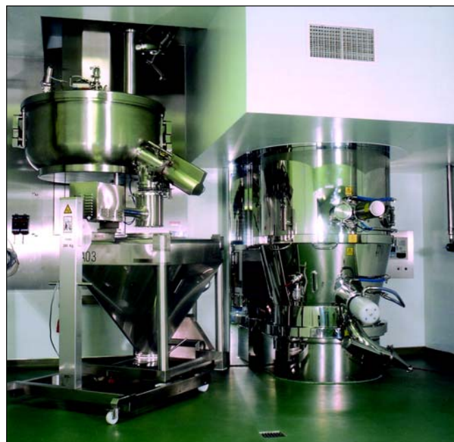
Figure 5. Granulation and fluid dryer suite.
