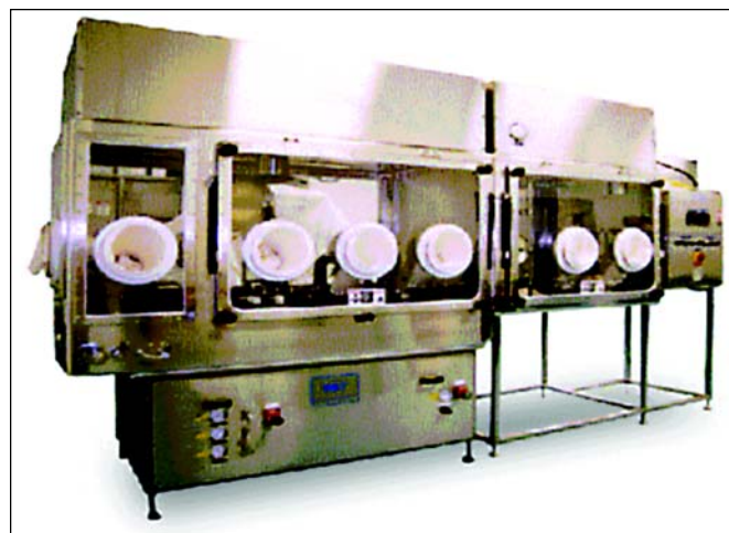
Figure 12. Class 100 high containment isolator system.
