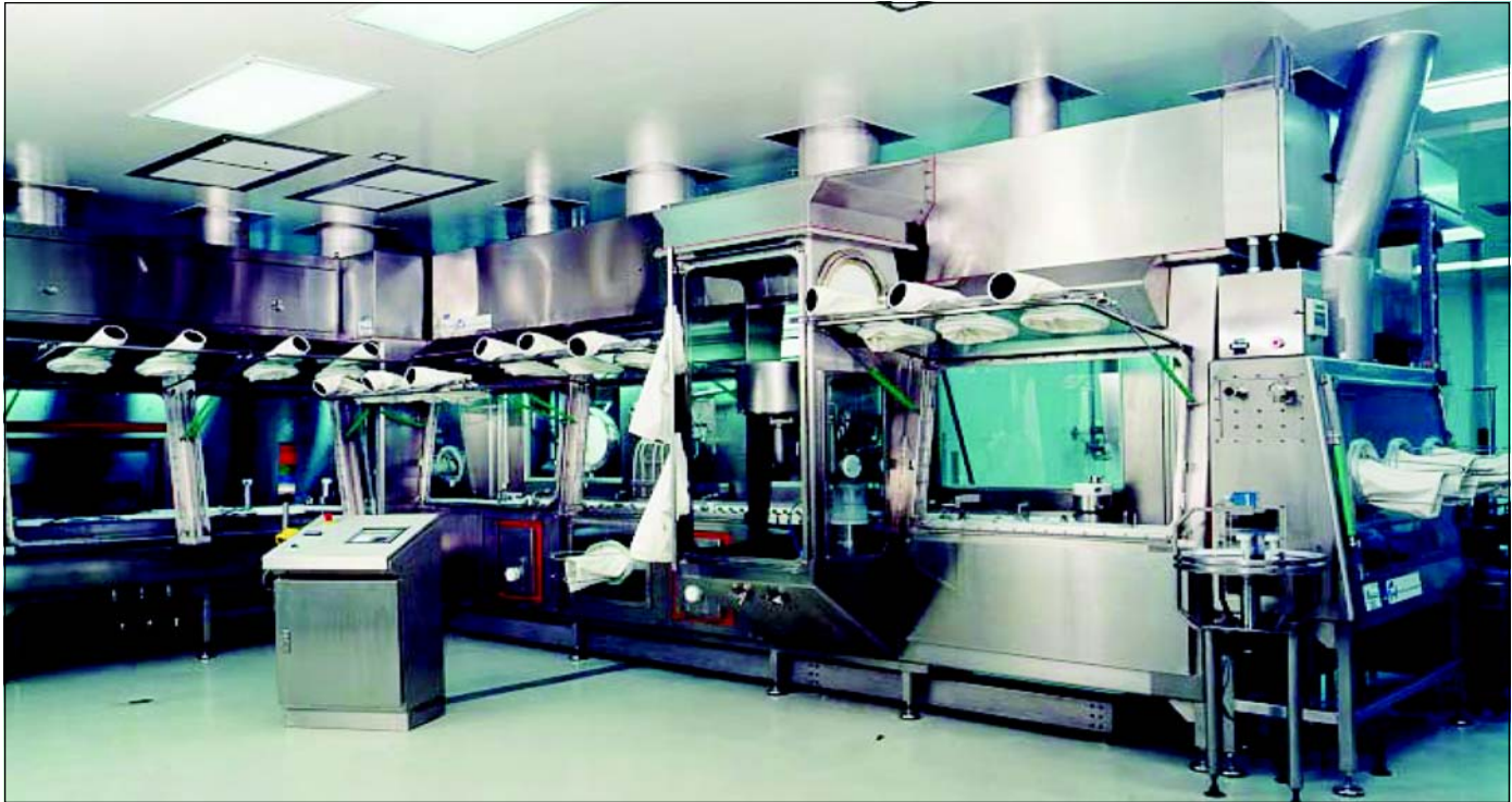
Figure 13. Isolated filling and lyophilizer operation.
