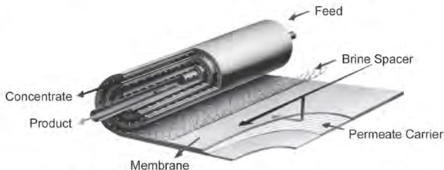
Figure 1. RO spiral membrane design.
