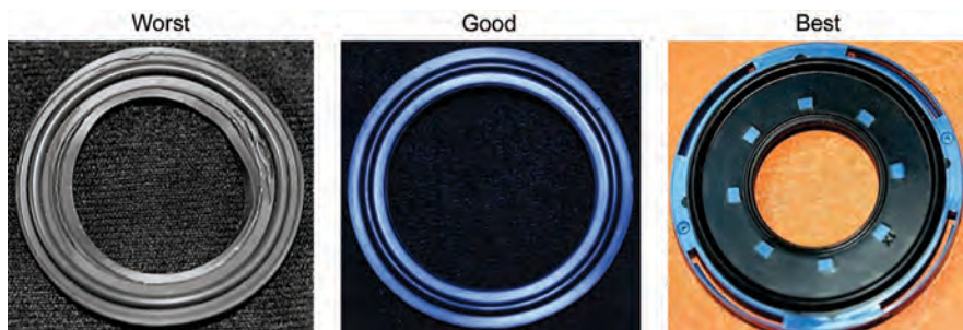
Figure 5. A range of gasket performance after 500 SIP cycles exposure (photos courtesy of The BioProcess Institute).
